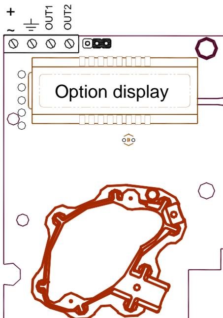
PCB with jumper to configure OUT2
