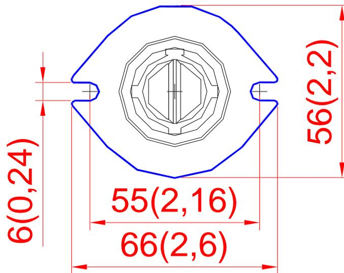
*The dimensions of the sampling probe in mm and (inches)*
